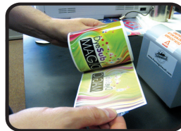
Step 4 Remove from press and peel transfer immediately for outstanding results.
