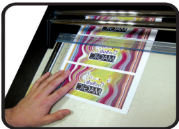
Step 1 Print Sublimation paper, in mirror image, then trim to size.
